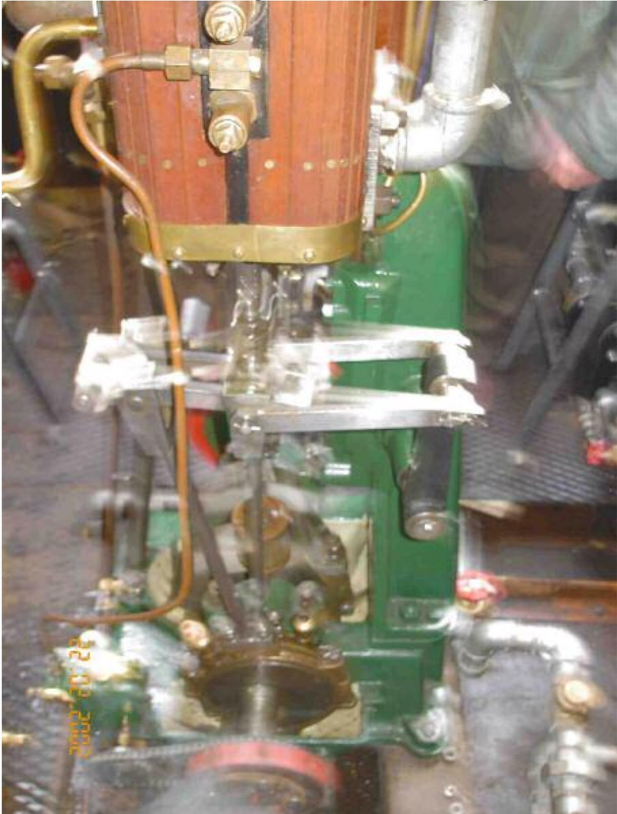
The new engine in steam and in motion. This picture is taken from the cabin looking towards the boiler. From the bottom the old baring wheel can be seen, with a chain drive to the lubricator. Just above this is one of the eccentrics. The engines green colour scheme and lovely wood and brass cylinder can be seen.
