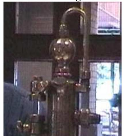
into water and displaces enough oil into the steam to lubricate the cylinder. Apart from being a wonderful piece of brass it is named the "Powell Half -Pint lubricator"!
