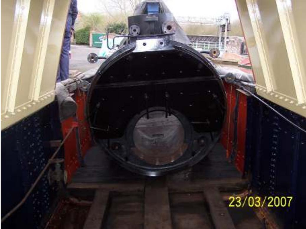
Once the boiler is located correctly all the bulk heads can be replaced and the work on connecting up all the pipe work can start.
