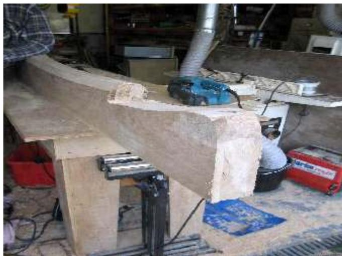
In this shot, the hole for the top hook has been drilled, and the top of the stock rounded over, ready for fitting the piece of aluminium to protect the end grain. Here the chamfers on the curved portion of the stock make sure the rudder does not foul Kildare's stern when on full lock. The preliminary shaping for the bottom hook and the bottom blade supports (floats ??) is also shown.
