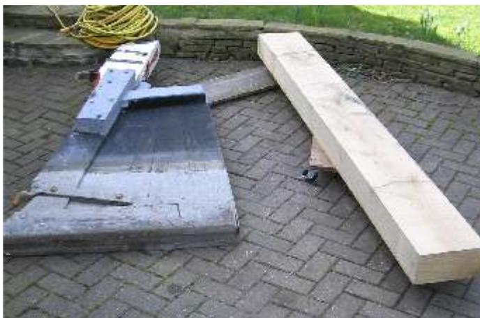
Timber for new rudder stock alongside old rudder showing mending plates after cracking last season
