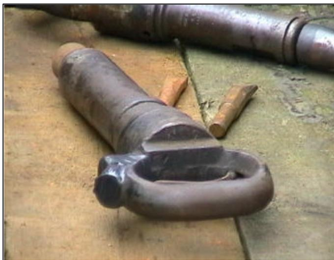
Pneumatic rivet gun ready for action. Photo Simon Nuttall
